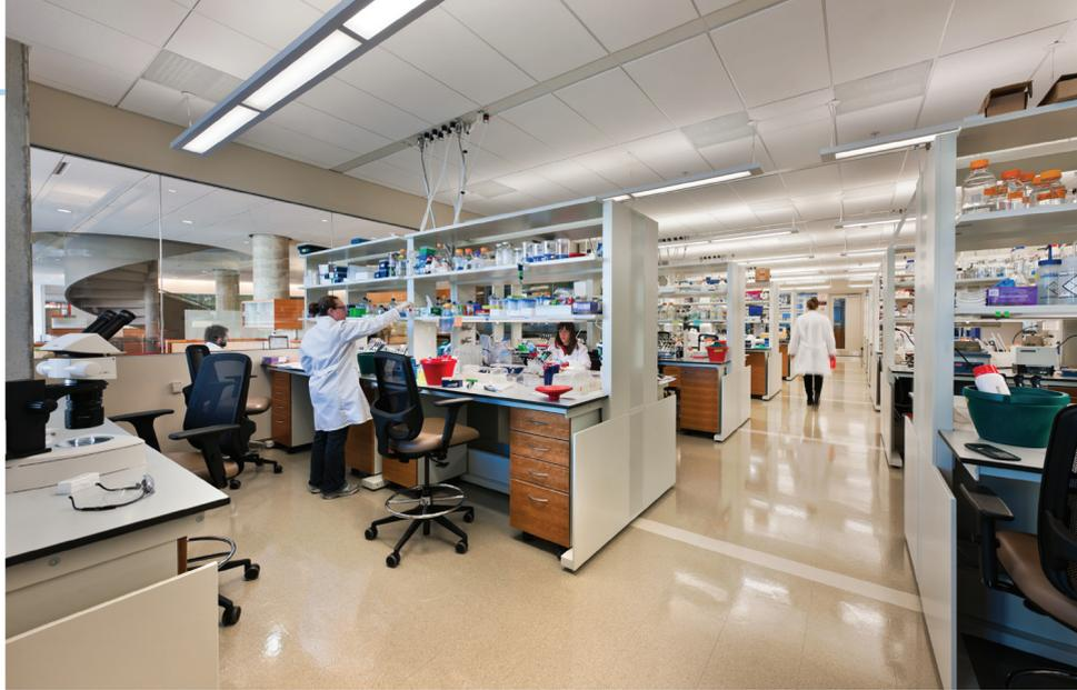
The wet laboratory pods for chemistry and biology are sized to accommodate interdisciplinary teams for up to five principal investigators. The laboratory furniture consists of rolling cabinets and 6-foot bench/shelving units that are moveable and/or removable for floor-mounted equipment. Photo: Tom Crane Photography
